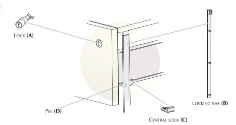
**2.** Opened pedestal. Turning the key **(A)** makes the locking bar **(B)** move downwards. Drawers can be opened without being impeded by the pins **(D)**.
