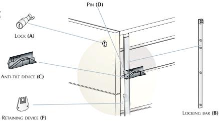
2. Opened pedestal. Turning the key (A) makes the LOCKING BAR (B) MOVE DOWNWARDS. DRAWERS CAN BE OPENED WITHOUT BEING IMPEDED BY THE PINS (D).
