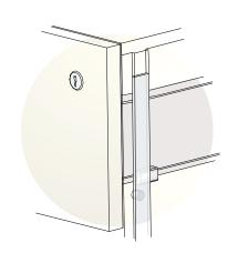
${f 3.}$  The opening of one drawer is not dependent on the locking bar (B), so all the drawers can be opened at the same time.
