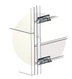
3. When opening one drawer, the anti-tilt device operates ON ONE PIN (D) MOVING THE LOCKING BAR (B) UPWARDS. THE RETAINING DEVICE (F) PREVENTS THE DESCENT OF THE LOCKING BAR (B) HOLDING THE PIN (E). THE REST OF THE DRAWERS CANNOT BE OPENED. THEIR RESPECTIVE PIN (D) IS PREVENTING THIS ACTION. When closing the drawer, the locking bar (B) descends ALLOWING THE OPENING OF ANY DRAWER.
