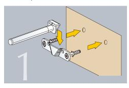
Place the support on the wall with the supplied wall plugs and screws and place the rod on the support.  $\hspace{-0.5cm}$
