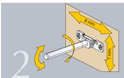
FIX THE SUPPORT IN ITS DEFINITIVE POSITION WITH THE OTHER TWO WALL PLUGS AND SCREWS TO AVOID THE SHELF DISPLACING THE LEVELLED POSITION.
